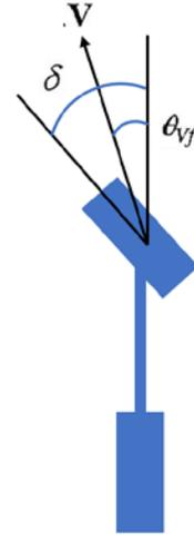
Figure 4 Description of tire slip angle in the two-degree bicycle model
