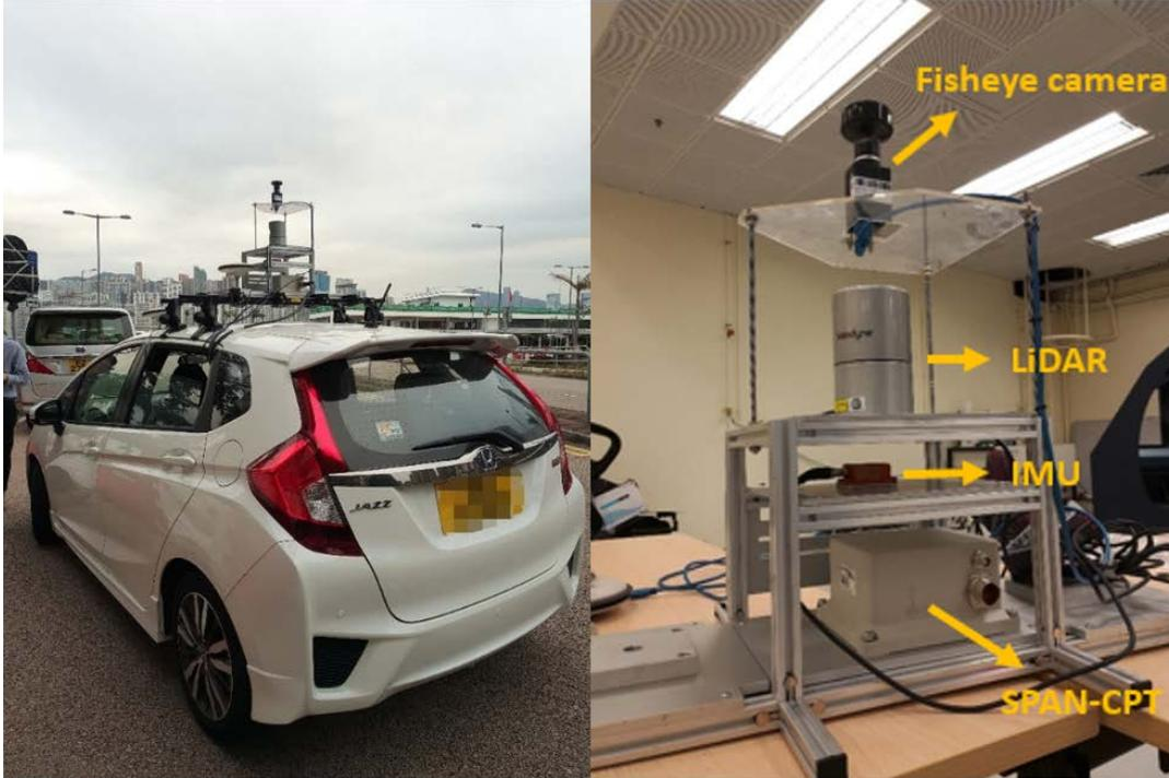
Figure 8 Data collection platform and sensors: including Fisheye camera, Velodyne 32E LiDAR, IMU and Novatel SPAN-CPT
